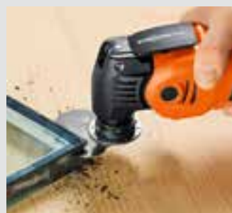
Separating insulating glass.
