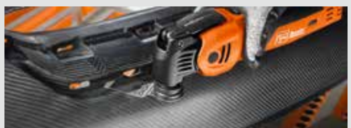
Cuts in carbon fibre materials.
