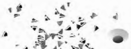
FINAL ASSEMBLY : With the ChipLet® feature, drill shavings are efficiently broken into small, easily evacuated pieces. The tools are available in different ergonomic shapes to give the best possible working conditions for the operator.
