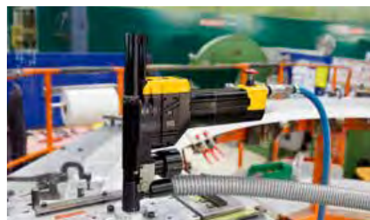
FINAL ASSEMBLY : With the ChipLet® feature, drill shavings are efficiently broken into small, easily evacuated pieces. The tools are available in different ergonomic shapes to give the best possible working conditions for the operator.
